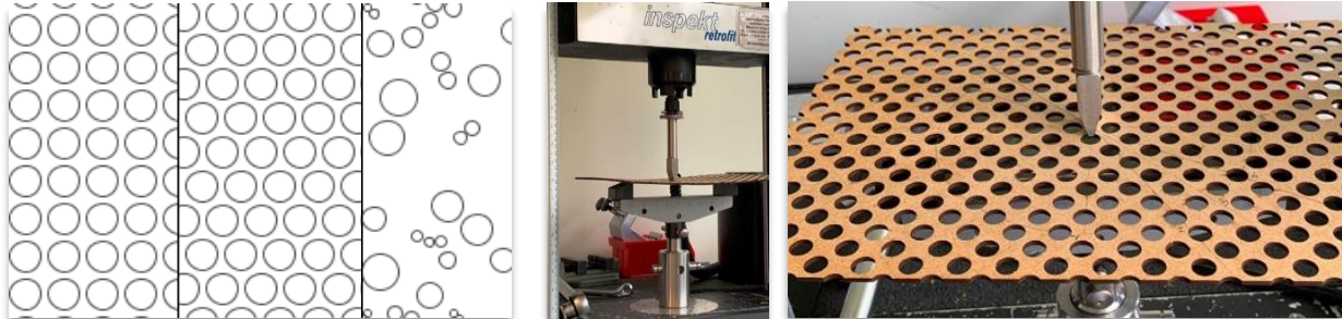
Fig. 1: Left: Three spatial arrangements of discs with different properties (two "regular" arrangements and one "irregular" arrangement). Center and right: 3-point mechanical bending test on an MDF wood plate lightened by circular holes.
